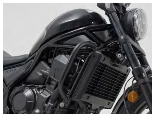
Crash bar - protection for the engine in case of overruns and falls
