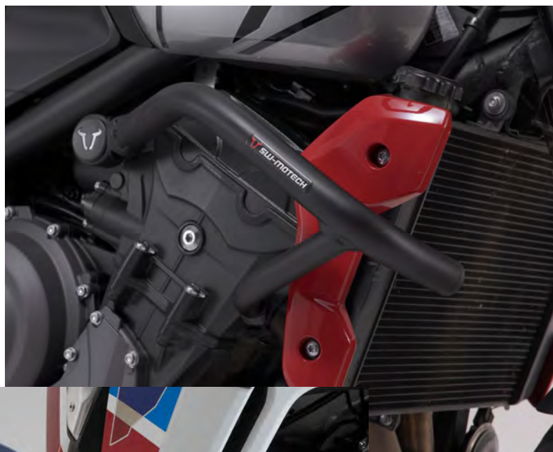
Left: Robust and discreet at the same time - Our crash bars for naked bikes
