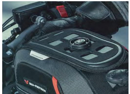
The T-Lock holder connects accessory bags with the MOLLE system by means of a twist lock
