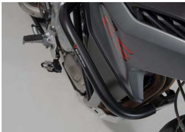
Right: Protection for the fairing by robust bars made of black powder coated steel
