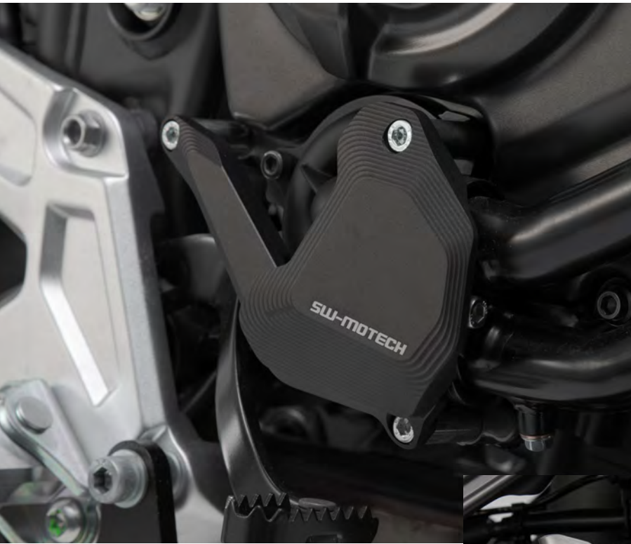
Water pump protection on the Ténéré 700 (left) and brake reservoir guard on the Africa Twin CRF 1100 (below)
