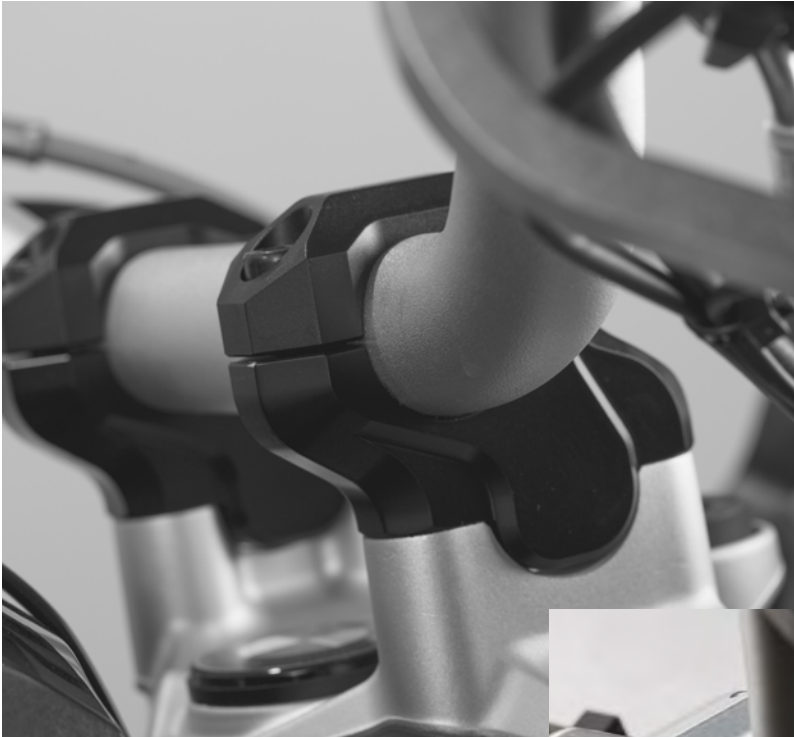
Handlebar relocations offer both: an increase of 30 mm and a relocation of 21 or 22 mm closer to the rider
