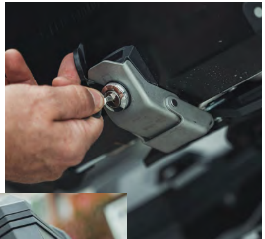
A lock in the latch buckle secures the top case against theft
