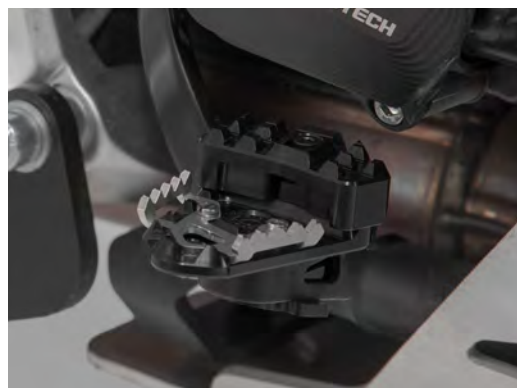
Two height settings for contact surface
