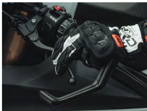
Protection for brake lever and clutch lever
