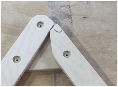
**Step 2:** Add the bolts to the 3 holes on the triangle and then push the legs together.
