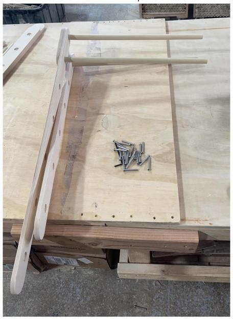
**Step 4:** Screw in remaining bolts and dowels to both the short and long leg.
