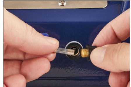
Step 3: Insert a new fuse, screw in the rotary knob
