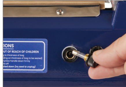
Step 2: Pull out the blown fuse
