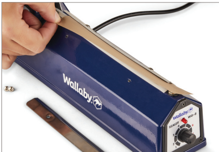
Step 1: Use tools to loosen the screws and remove the cover and cloth
