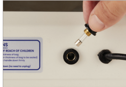
Step 2: Pull out the blown fuse
