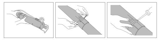
**10.** Place the Front Duct Assembly (7) onto the Mid Duct Assembly. Slide the long screw into the slot between the two sections and secure it into the remaining nut with a Phillip's head screwdriver.
