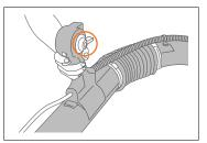
**3.** Simply hold down the trigger to activate the Vortex<sup>™</sup>. The trigger can be locked on the ON position using the switch on the side of the handle (circled).
