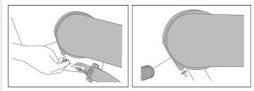
**5.** Slide the washer onto the U-Clip where the threads protrude from the slot below.
