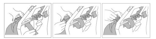
1. Bring the ComfortStraps<sup>™</sup>(4) to the bottom of the Lower Housing (5). Attach the strap clips to the loops on the housing. 2. Take the top of the ComfortStraps<sup>™</sup> and slide it through the loops at the top of the Main Housing. Feed the strap under and over the strap buckle. Gently tug on the strap to tighten in place and ensure it is secure.
