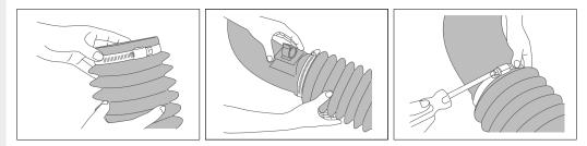
**7.** Place a Clamp (10) over one end of the Bellows Duct (8). Place it over the opening of the External Elbow Duct. Tighten the Clamp using a screwdriver.
