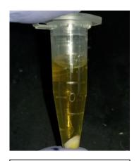
The sample was centrifuged at 14,000xg and 0.22  $\mu m$  filter prior to injection into the HPLC.
