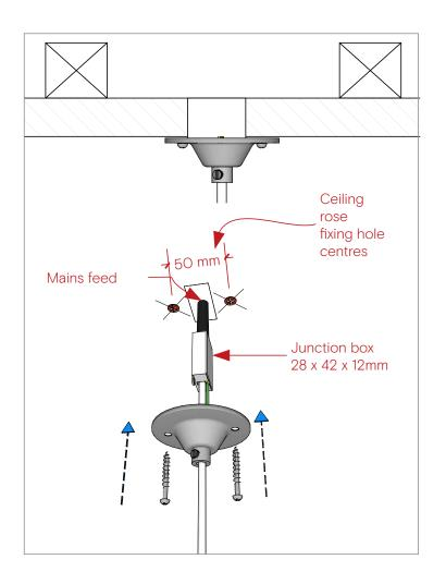
Bracket with side fix Wiring connection contained in ceiling rose.
