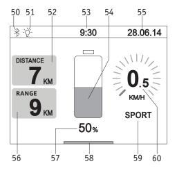
When the control unit is switched on, the Alber start screen (if activated) appears first and after about 3 seconds this changes to the user screen illustrated in the adjacent diagram. The diagram shows all the symbols that can be shown on the control unit display.
