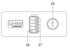
5 LEDs light up – the battery pack is charged to 100%. Avoid high speeds when driving down slopes as the current feedback in the wheels may lead to overvoltage in the battery pack and force the wheels to shut down.
