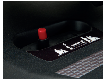
Two step disengaging lever prevents the scooter from accidentally free-wheeling.
