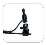
Very small profile joystick ideal for chin control due to the outer shell being resistant to saliva and other foreign objects. Comes with a headrest and an egg switch for function and profile changes. Its built in Bluetooth allows simple access to computers or communication devices.
