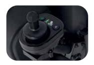
Allows access for up to three drive functions and all seating functions with graphic display, attendant in charge indicator and status LED's.
