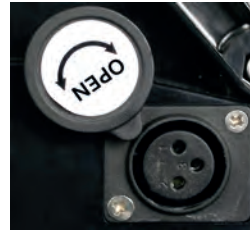
(I) CHARGING DOOR OPEN
