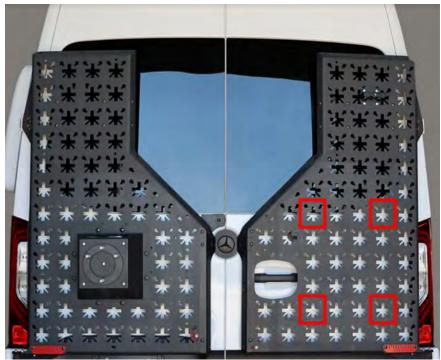
4. Install the handEtrack hardware (A) into the nVader rack. Loosen the center screw until it is nearly removed. Slip the back portion of the handEtrack into the vertical slot, and align it to be centered up and down. Tighten the center screw to hold in place.
