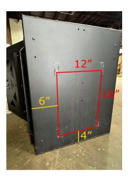
2. Drill a 3/8" hole at each of the four marked locations.
