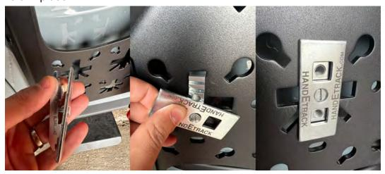
5. Place a lock washer (D) and sealing washer (C) on all four bolts (B). The sealing washer should be facing out so that it contacts the sheet metal surface of the box as shown below.
