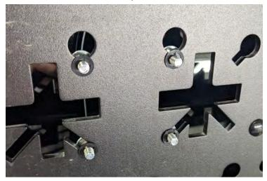
4. Place all four bolts from Step 2 into the slots on the nVader rack.
