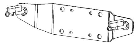
2. Place retaining washers (C) on all four carriage bolts (A), leaving space for the thickness of the nVader rack.
