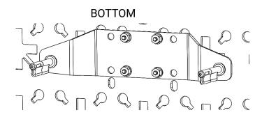
5. Place traction boards on the mounting pins and rotate the pin ends to secure. We Strongly recommend adding security locks to pins to deter theft.
