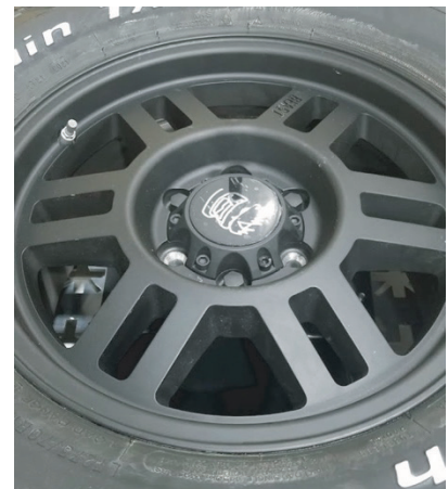
Figure 9 Install (4) lug nuts.
