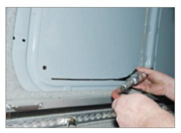
5. Apply a bead of supplied 3M adhesive to the glue flange of the part. Leave about 1/2" space to the outer edge and apply an even bead. Shape it to a triangle as shown in the video, this will reduce the need for clean-up.
