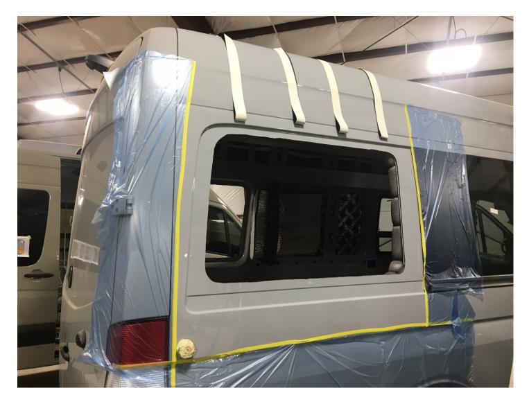
3. Remove the rear quarter panel by cutting along the factory window edge. Prime the cutline to prevent rust.
