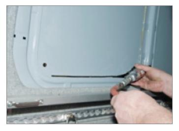
5. Apply a bead of supplied Loctite 5555 adhesive to the glue flange of the part. Leave about 1/2" space to the outer edge and apply an even bead. Shape it to a triangle as shown in the video, this will reduce the need for clean-up.
