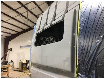
the tip of the caulking gun. Skipping this step can cause pin holes and water leaks!
