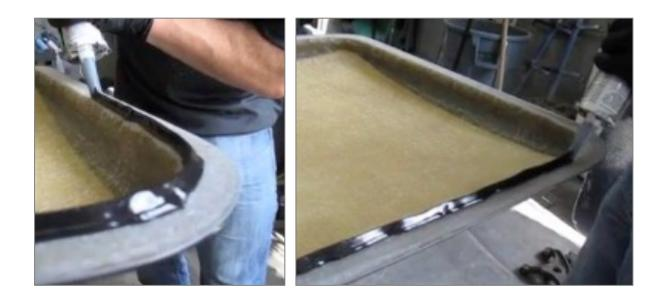
6. Install the flare by lining up the top edge of the flares and your vertical tape mark then slowly set the flare into the indentation of the rear quarter panel, making sure you are lined up with the OEM radius top and bottom, leaving 1/16" space. One person will hold the part in place while the second installer firmly presses the glue flange onto the van.
