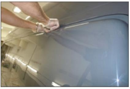
8. Secure the part with strips of masking tape for a min of 12 hours. Tip - gaffer's tape works best!
