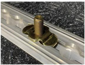
The Threaded bolt sits in between the circles along the L-track and the lock washer ends sit inside the circles. The lock washer prevents the threaded bolt from moving out of place while driving.
