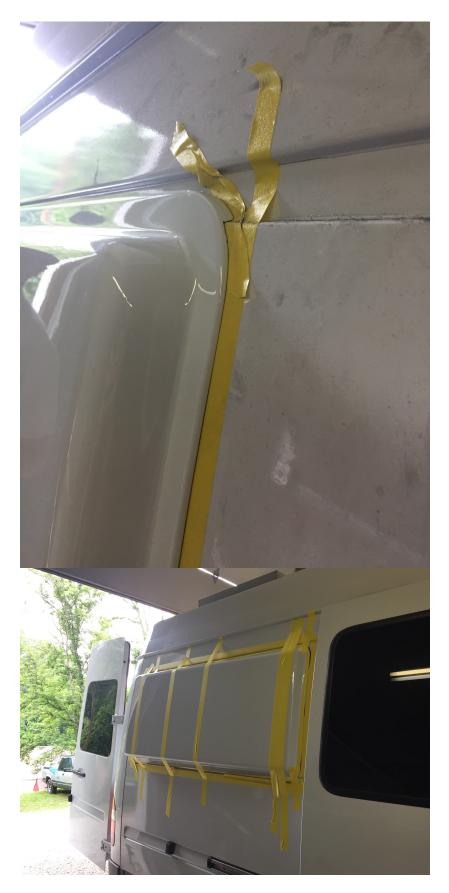
The glue flange will now sit inside the channel and is notched along the front leading edge.
