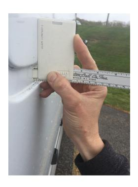
Build a test block out of wood to get the exact shape off the van for the front leading edge of the flare. Knowing the depth and width of the channel will allow you to set your router correctly.
