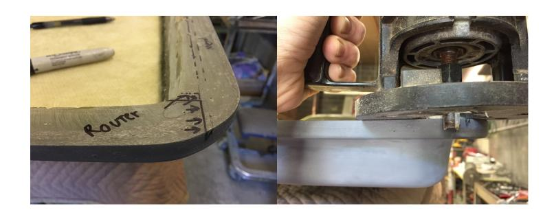
Router out the front leading edge of the flare, leaving 1/8" of material. Test fit repeatedly as you remove material.
