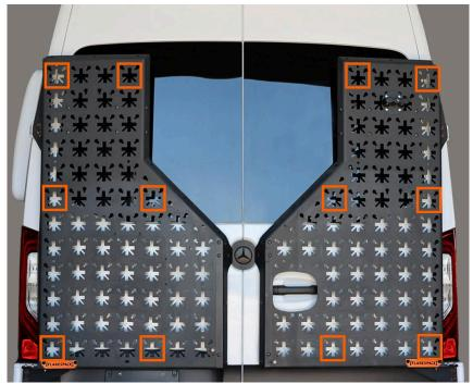
3. Install the handEtrack hardware (A) into the nVader rack. Loosen the center screw until it is nearly removed. Slip the back portion of the handEtrack into the **VERTICAL** slot, and align it to be centered up and down. Tighten the center screw to hold in place.
