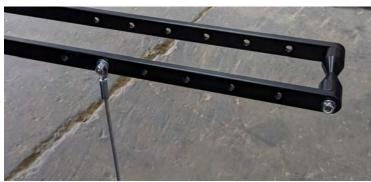
7. Place a carriage bolt (A) through the flat side of the eyelet (F) as shown below, and secure loosely with a Nylock Nut (B). With the 1UP arm horizontal, place the carriage bolt through the highest possible 1/4" slot in the NVader Rack and tighten with a 7/16" Wrench.
