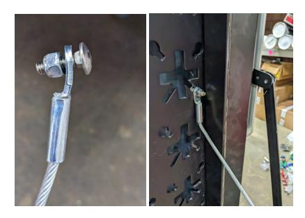
8. Lower the arm of the 1UP Rack until the cable is snug. The final position of the 1UP Arm should be slightly above horizontal. Adjust the position of the carriage bolt from Step 6 if necessary.
