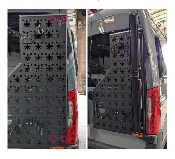
6. Lower the bottom arm of the 1UP rack until it is slightly above horizontal. Attach the following hardware in order through the 2nd hole in the arm of the 1UP rack. This hardware should be placed on the side opposite of the levers on the 1UP rack. Tighten until the cable is snug but still able to rotate.
