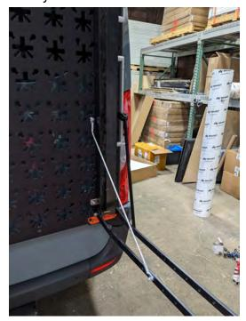
9. The rack is now ready to use. Fold arms closed when not in use. When transporting a bicycle, use the included voile strap to secure the top wheel to the 1UP rack.
