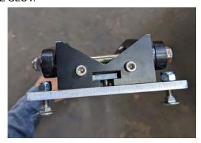
4. Place the first bracket 1.5 inches from the end of the 1up rack. This will be the lower end of the rack. Place the second bracket so that the two brackets have 43 inches in between each other, and tighten bolts with a 4mm Allen Wrench.
