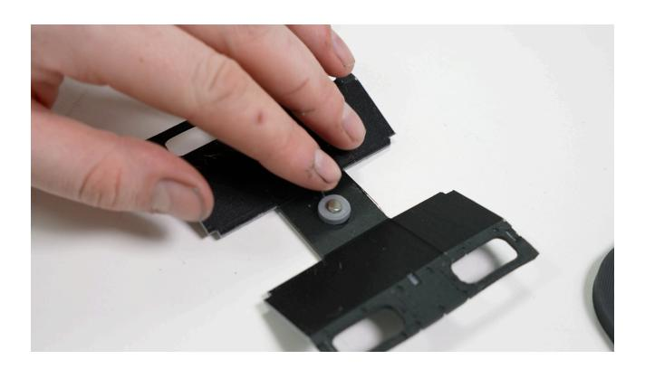
STEP 2: Place the arm holder in the square slot in the lid. Make sure that the motor is facing the top of the lid. Then secure with the M2.5x6 screw.
