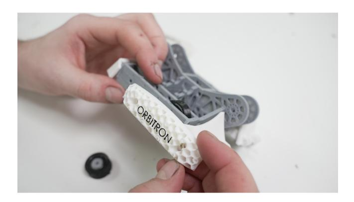
STEP 5: Insert a M3x25 screw through the assembly.
