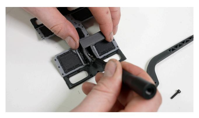
STEP 3: Insert the arm into the arm holder and secure it with the M2.5x12 screw.
