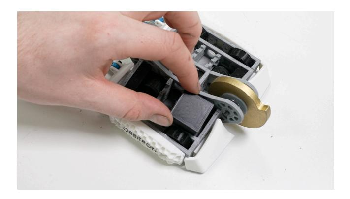
STEP 4: Insert the drive motor into the long narrow section of the frame, with the square side facing the wheels. Secure with a drop of superglue. Repeat for the other side.
