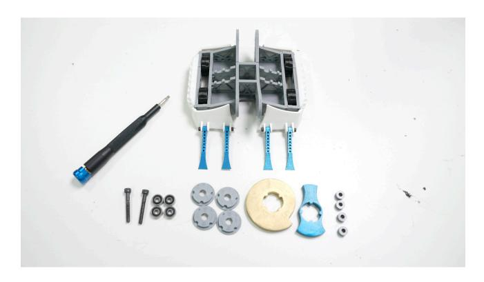
STEP I: Insert the 604 bearings into each of the 4 spinner bearing holders.
