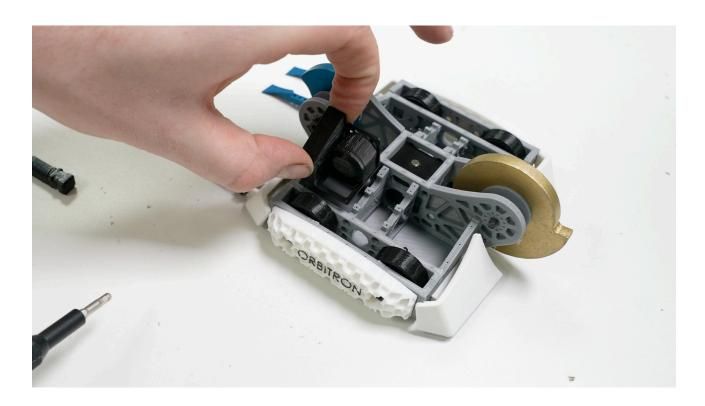
STEP 3: Insert the batteries into the remaining two corners and secure with a drop of superglue.
