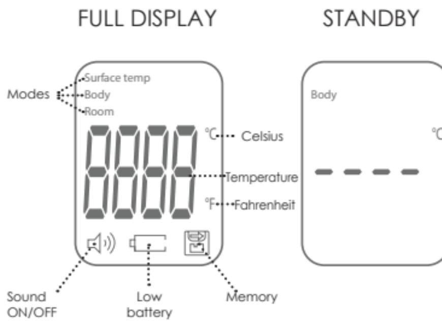
2. Press the °C/°F Button to select the desired temperature unit.
