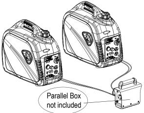
**Note:** Most electronic devices require power beyond its rated wattage to start. This additional power is referred to as surge watts and usually lasts between 2-3 seconds. When an electronic device is started, the red overload indicator may come on. This is normal. If the light stays on disconnect all electronic devices and stop the engine. Refer to "Engine Overload Indicator Light" on page 8.
