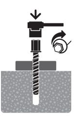
Install with either a socket or cordless impact driver. Apply pressure against the fixing and rotate to engage the first thread
