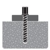
Continue to tighten the anchor until flanged head is firmly seated against fixture. Installation complete!
