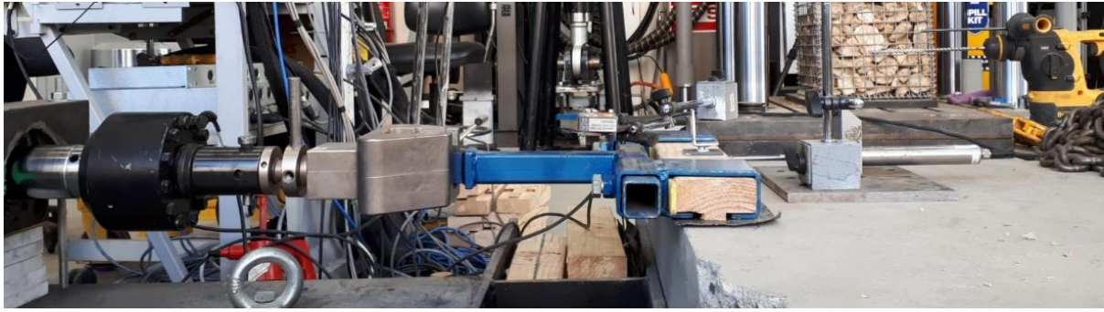
Figure 11: Out-of-plane shear test setup
