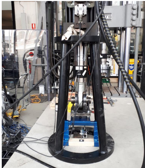
Figure 5: Test setup and instrumentations for tension test
