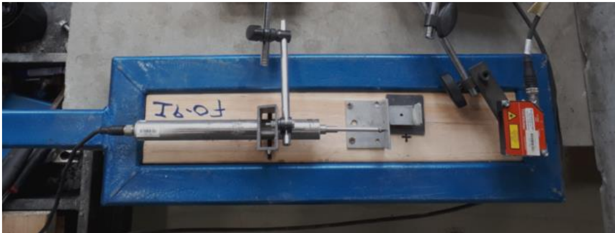
Figure 9: Close up view of the in-plane shear test setup
