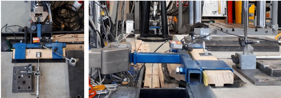
Figure 12: Close up view of the out-of-plane shear test setup
