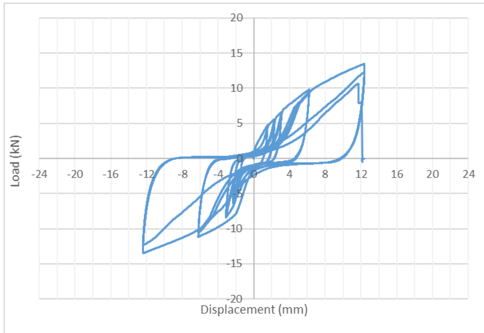
Figure 23: Load displacement curve for in-plane shear test #3
