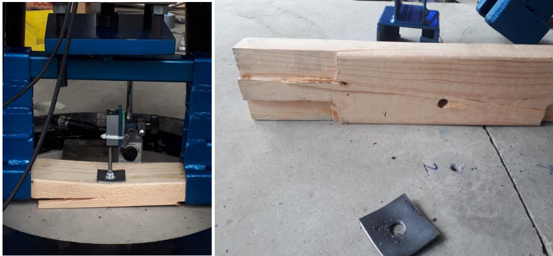
Figure 13: Bottom plate timber failure
