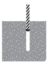
Using a 10mm drill but, drill a hole to the depth of at least one diameter deeper that the required embedment depth.
