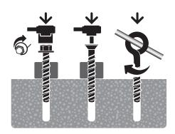
Install with either a socket or cordless impact driver. Apply pressure against the fixing and rotate to engage the first thread. Continue to tighten the anchor until flanged head is firmly seated against fixture.
