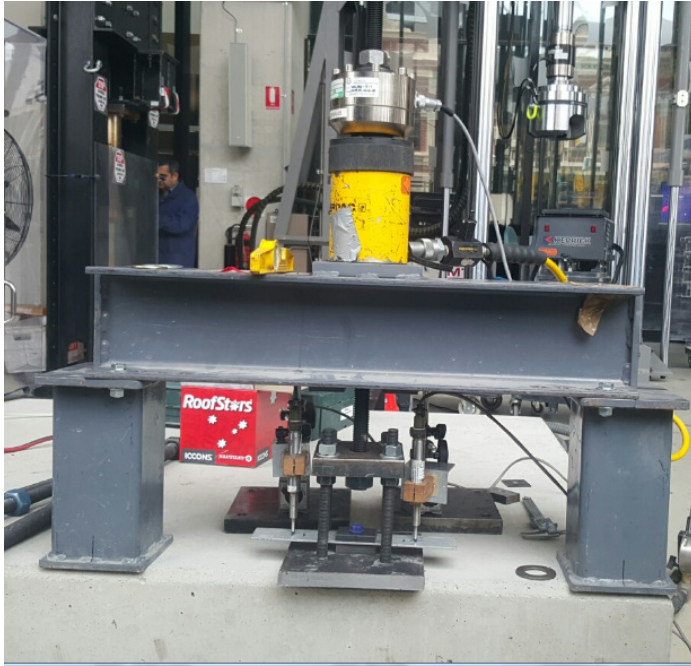
Figure 4: Test setup and instrumentations for tension test
