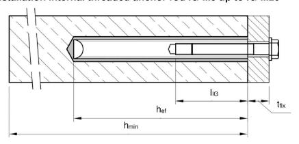
$t_{fix}$  = thickness of fixture
