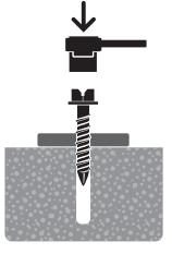
Install with either a socket or cordless impact driver. Apply pressure against the fixing and rotate to engage the first thread.
