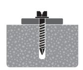
Continue to tighten the anchor until hex head is firmly seated against fixture. Installation complete!
