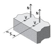
To achieve published tension and shear loads the anchors should be installed at least 12 x the anchor drill diameter between each other. If spacing between anchors is closer than 12 x the anchor drill diameter apply appropriate reduction factor as outlined in the SPACING TABLE to the published load to ascertain the reduced load.
