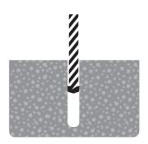
With the correct diameter drill bit, drill a hole to the depth of at least one diameter of the anchor deeper than required embedment.
