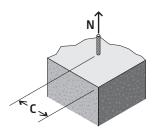
To achieve published tension loads the anchors should be installed at least 8 x the anchor drill diameter from a concrete edge. If edge distance is closer than 8 x the anchor drill diameter apply the appropriate reduction factor as outlined in the EDGE DISTANCE TENSION TABLE to the published load to ascertain the reduced load.
