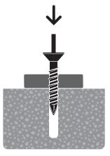
Install with either a socket hex driver or cordless impact driver. Apply pressure against the fixing and rotate to engage the first thread.
