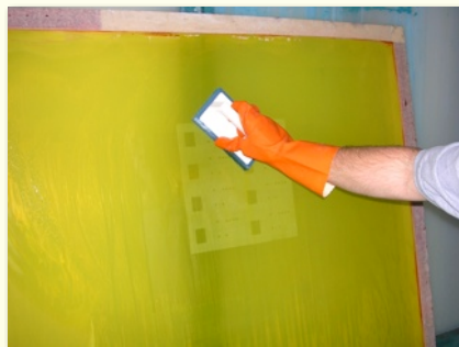
Step 2. Scrub screen with non-abrasive pad or brush. Allow screen to dwell up to 10 minutes.
