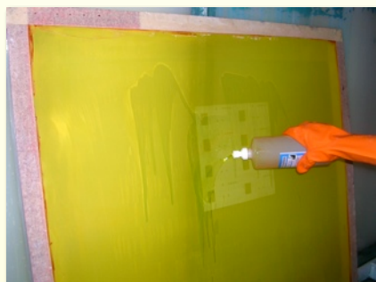
Step 1. Apply RE-STOR to both sides of the screen.
