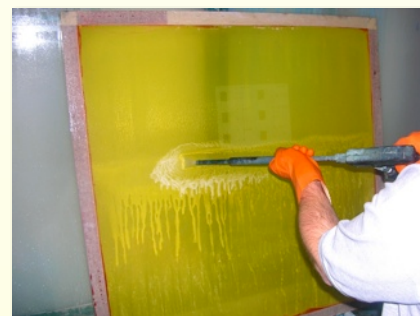
Step 3. High pressure rinse - starting at bottom.
