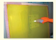
Step 1. Apply LSR-30 to both sides of a wet screen.
