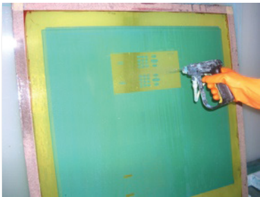
Step 1. After removal of ink, block-out, and tape, apply CDR-Concentrate® to a wet screen (both sides).
