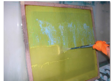
Step 3. High pressure rinse - starting at bottom.
