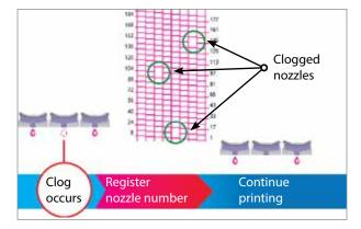
If a nozzle clog is not cleared via the maintenance function, other nozzles can be assigned to continue printing. Print speed is largely unaffected.
