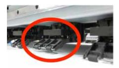
Operators can manually push down on the lever (above left) when the pinch roller is in the down position to raise it off the media (above right).
