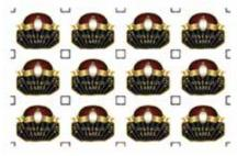
A maximum of four crop marks are automatically and continuously detected so printed images are accurately cut.
