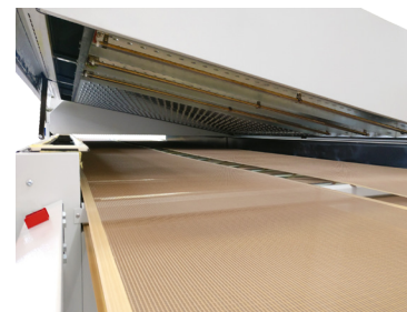
Infrared Lamps and upper section opening
