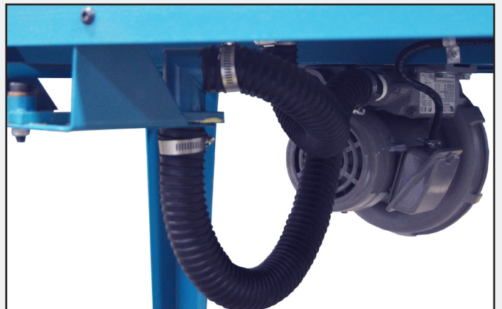
The Accu-Glide features a heavy-duty Max-Air Vacuum Motor standard.
