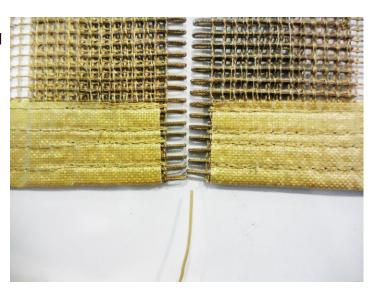
• Be careful to joint the belt in the correct position without losing any hooks. The edge must be flat and without any indent.
