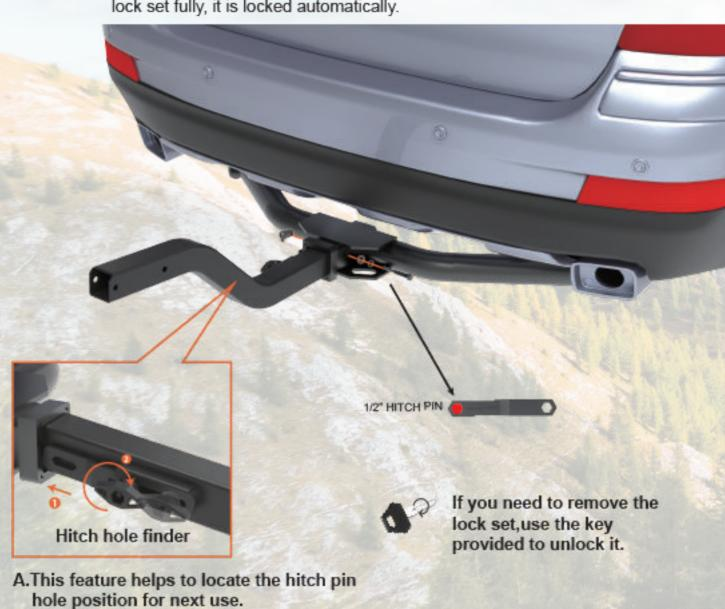
B.Once you tighten the knob, it automati cally locates the hole for next hitch pin insertion.
