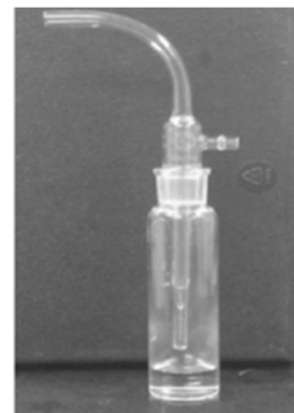
Figure 5: AGI-30 impinger used for bioaerosol sampling during trials
