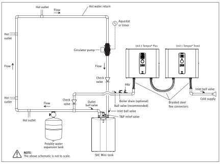
If necessary, installing 2 Tempra® units will increase flow rates. Split temperature rise desired between units. Example: Unit 1 set to 90 °F (32 °C) & Unit 2 set to 115 °F (47 °C).
