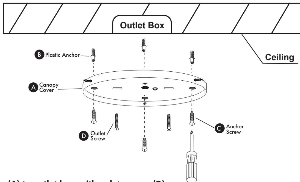
Attach canopy cover (A) to outlet box with outlet screws (D). Screw anchor screws (C) into plastic anchors (B) to secure canopy cover (A).
