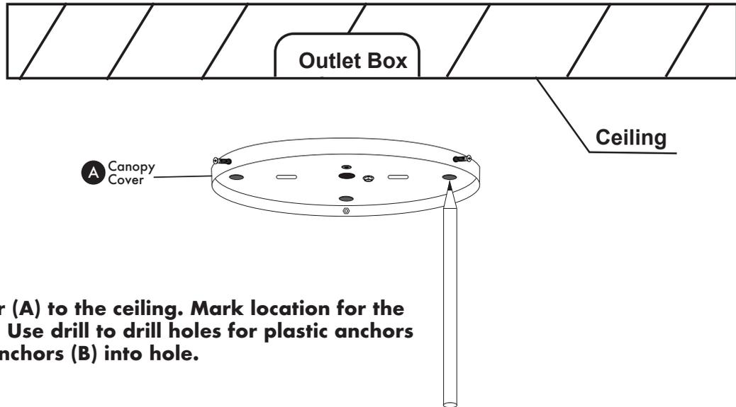
Raise canopy cover (A) to the ceiling. Mark location for the plastic anchors (B). Use drill to drill holes for plastic anchors (B). Insert plastic anchors (B) into hole.
