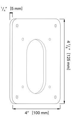
For retrofits. Great for brick and stucco and many siding types. Plate extends the mounting screws further from the entry hole—perfect for crumbling masonry or covering larger entry holes. Hydrant attaches to the mounting plate with included machine screws.
