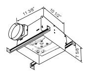
STERLING ventilators come with permanent split capacitor motor, which improves efficiency and enables the STERLING line to carry the ENERGY STAR label.
