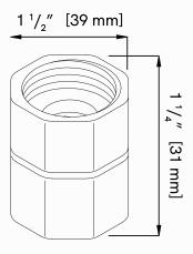
Use the stainless steel Double Female Hose Adapter to handily connect two male garden hose ends together. It works great for our RV City Water Inlet, or any situation where Aquor hydrants are used as fill valves.
