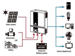
Figure 1 Basic hybrid PV System Overview
