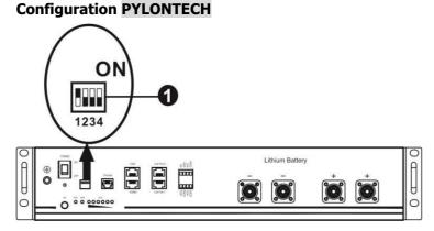
①Dip Switch: There are 4 Dip Switches that sets different baud rate and battery group address. If switch position is turned to the "OFF" position, it means "0". If switch position is turned to the "ON" position, it means "1".
