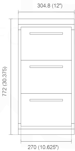
. MIDDLE CABINET - FRONT ELEVATION
