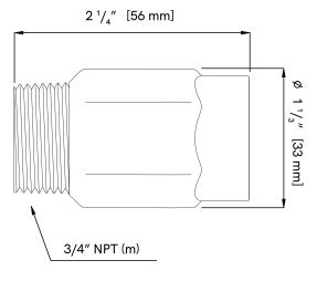
This inlet replaces the default hydrant 1/2" NPT inlet. Adapts to larger 3/4" plumbing. Use with any plumbing - NPT is the most common thread type.
