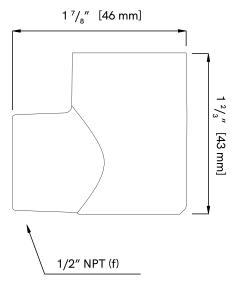
For a more flexible installation, replace the standard straight hydrant inlet with this  $90^{\circ}$  elbow. The elbow inlet shortens the overall length of the hydrant by 1/2''. Use with any plumbing - NPT is the most common thread type.
