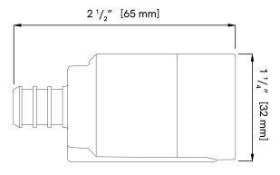
This inlet replaces the default hydrant 1/2'' NPT inlet. Quickly and reliably connect your Aquor hydrant to 1/2'' PEX tubing with a crimp connection.
